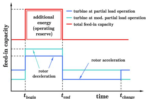
Fig. 4 Idealised process of providing control reserve
