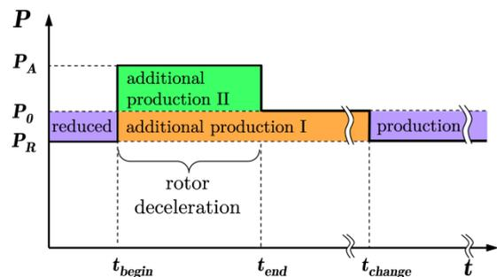
Fig. 3 Additional power and reduced power at modified partial load
