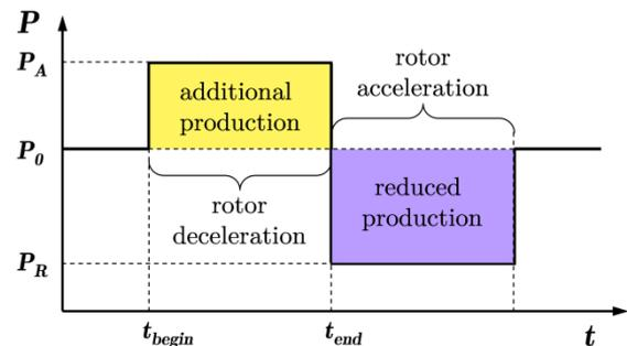
Fig. 2 Additional power and reduced power at partial load
