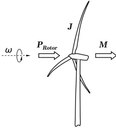
Fig. 1 Model of the rotor dynamics
